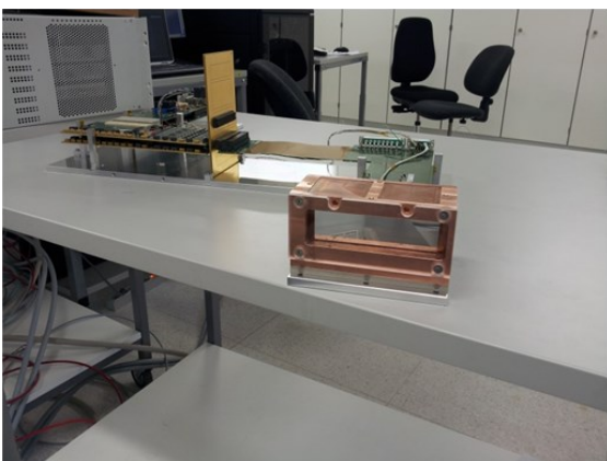
Figure 1. A single 128 x 512 pixel tile of the AGIPD system
